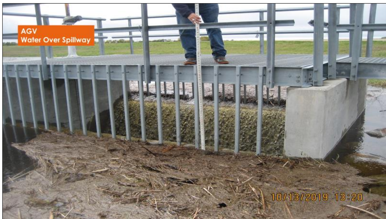
Technician Danny Omdahl is pictured measuring the amount of excess water overflowing the spillway at Agassiz Valley Impoundment site this past fall.
