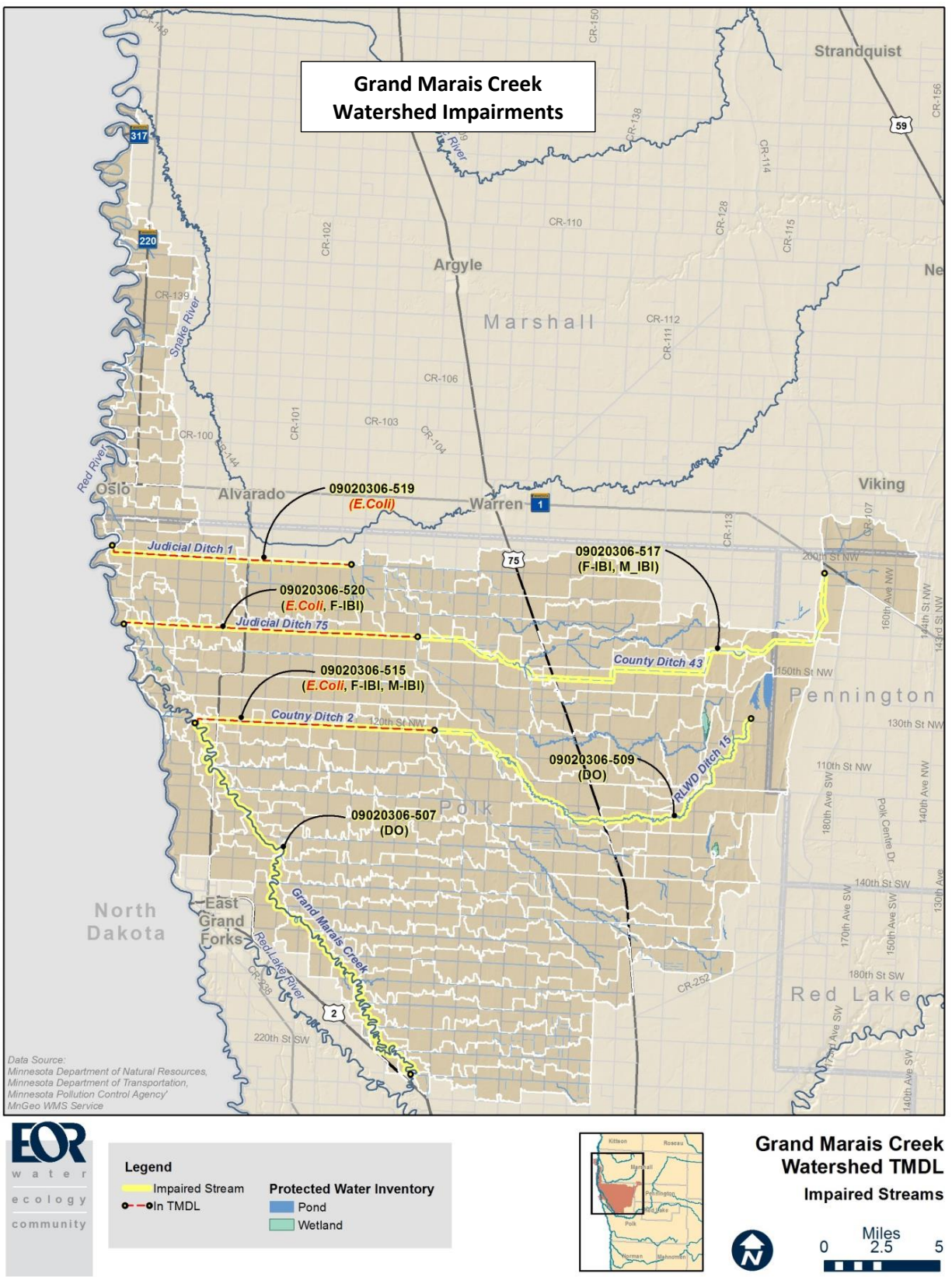
Figure 1-1. Impaired streams in the Grand Marais Creek Watershed addressed by this TMDL
